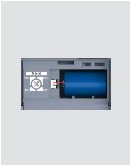
Open the battery flap to access the neutral protection dial. Thanks to the battery, the tripping cause is displayed on the screen after a trip.
