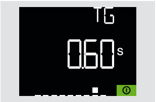
Ground fault delay setting.
