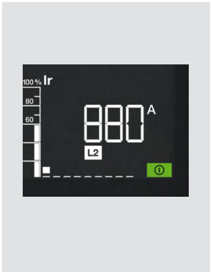
Each parameter is displayed in real-time, in amps or seconds. You can set all long time delay, short time delay, and instantaneous protection parameters, and depending on your product customisation, either the neutral protection or the ground fault protection.
