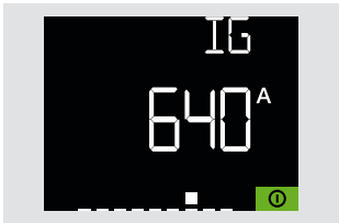
Ground fault threshold setting.
